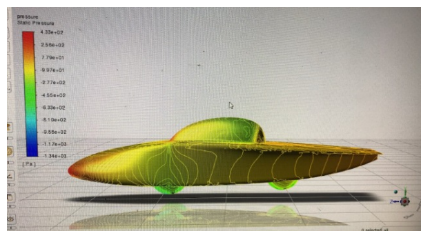
Figure 2: Pressure distribution over custom airfoil profile. Blue regions indicate low pressure (suction) while red shows high pressure zones. The gradient visualization validates laminar flow characteristics and separation point optimization for minimum drag.
